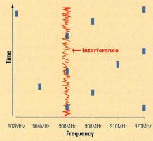
In frequency-hopping spread spectrum (FHSS) radio, the signal spends only a small amount of time on any one frequency in the spectrum. By making the signal hop from one frequency to another, the transmitters increase their immunity to interference in the spectrum.
