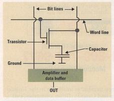
Figure 2: A simple 1-bit DRAM cell consists of a capacitor and a transistor. A charge in the capacitor represents a 1, while a lack of charge represents a 0. Applying a voltage to the word line closes the transistor, connecting the capacitor to the right-hand bit line. This produces a small voltage difference between the left and right bit lines and results in the cell's value being read to the output line.
