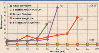
FAIL-The wireless LAN system failed to complete the test at d
