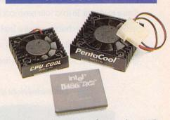
It's a fact. 486 chips run hot, often exceeding 185°F! Now, you can cool your 486 to a safe 85°-95°F with our popular CPU-Cool. Consists of a long-life ball-bearing mini-fan inside a die-cast heat sink that easily mounts on the CPU. Powered by a spare drive connector. Effective, inexpensive insurance!
