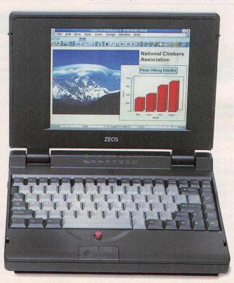
The 800C includes a generous 10.3" dual-scan color backlit screen for easy viewing (9.5" active matrix display is also available); two Type II or one Type III PCMCIA slots; and an internal 3.5" 1.44MB floppy drive.
