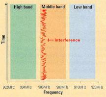
Direct-sequence spread spectrum (DSSS) transmitters transmit the signal over a specific band of the frequency spectrum. The signal does not hop around to avoid interference as it does with FHSS. To minimize data loss from interference, the transmitter adds redundant bits, or chips, to the signal, so that it retains enough bits to make it safely to the receiver.
