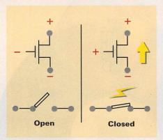
Figure 1: A transistor in a computer circuit acts as a miniature switch, controlling the flow of electrons from one location to another. Applying a voltage to the transistor closes the switch and completes the circuit, while removing the voltage opens the switch and shuts off the flow of electrons.
