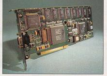
DOUBLE THE FUN: Number Nine's Imagine128 video card features a widebandwidth 128-bit accelerator chip.
